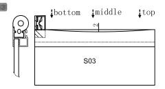
Put the glass on the ground, silicone the vertical profile on the glass, and press the middle part of the vertical profile and let the profile completely touch the glass; press slightly in the top and bottom part of the vertical profile, leave around 2mm space between the glass the vertical profile
